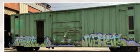
ARRC converted a boxcar into a Geometry Car that can measure track features and detect defects, to better plan track maintenance.
