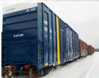
ARRC converted a boxcar into a Geometry Car that can measure track features and detect defects, to better plan track maintenance.
