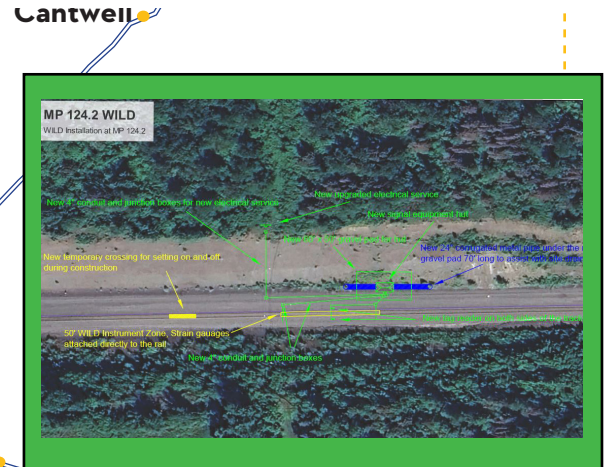
Photo above details MP 124.2 wheel impact load detector (WILD).
