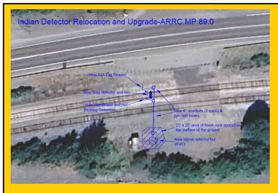
The detector site currently located at MP 88.7 (near Indian) will be relocated to MP 89.0 and receive upgrades to its talker and dragger.
