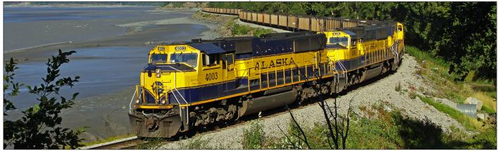
SD7OMAC locomotives haul coal-filled hoppers from the Healy coal mine to the loading facility in Seward. (photo by Frank Keller)
