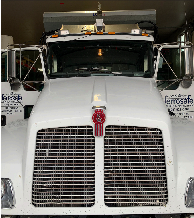
The Ricospray infrared camera is mounted on top of the Ferrosafe truck cab, to provide a clear vantage point for detecting weeds.
