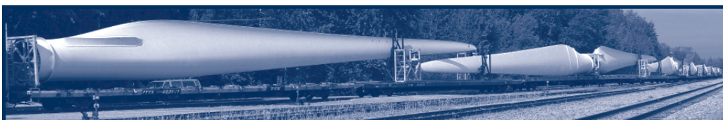
Two 149-foot wind turbine blades fit onto three flat cars. (Photo by David Blazejewski).
