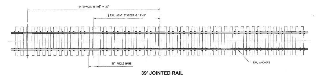
FOR 39' JOINTED RAILS IN MAIN LINE TRACK, 24 TIES AND 40 RAIL ANCHORS PER RAIL, 3250 TIES, 5416 RAIL ANCHORS, 272 PAIRS OF ANGLE BARS, AND 1632 ANGLE BAR BOLTS, NUTS AND WASHERS PER MILE
