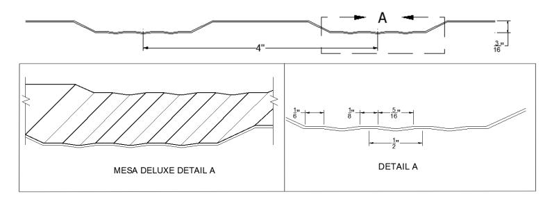
The mesa panels provide a 36-inch durable wall coverage with a ridged, S-lock panel joint. As shown in detail A, the mesa deluxe panel, is profiled with two minors centered between the major rib, while the mesa panel is profiled with 3/16" tall ribs and flats. Either panels are available in both zincalume and pre-painted zincalume coated steel. The paint coating consists of a high quality Silicone Modified Polyester (SMP) finish in the colors listed below:
