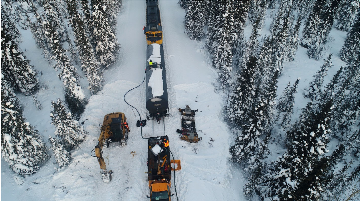
Alaska Railroad crews empty Jet A fuel from a derailed tank car on Thursday, Jan. 17. The transferred fuel was later transported to Fairbanks.
