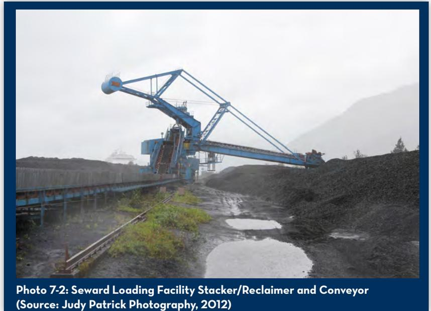
**Photo 7-2: Seward Loading Facility Stacker/Reclaimer and Conveyer**
