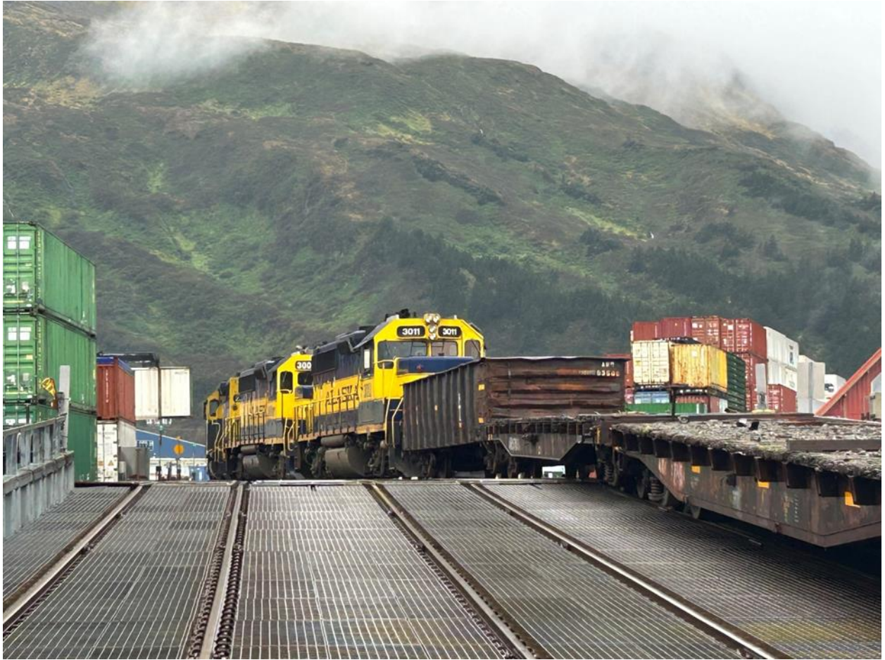
Figure 7. Inbound train shoving idler flats onto transfer span.
