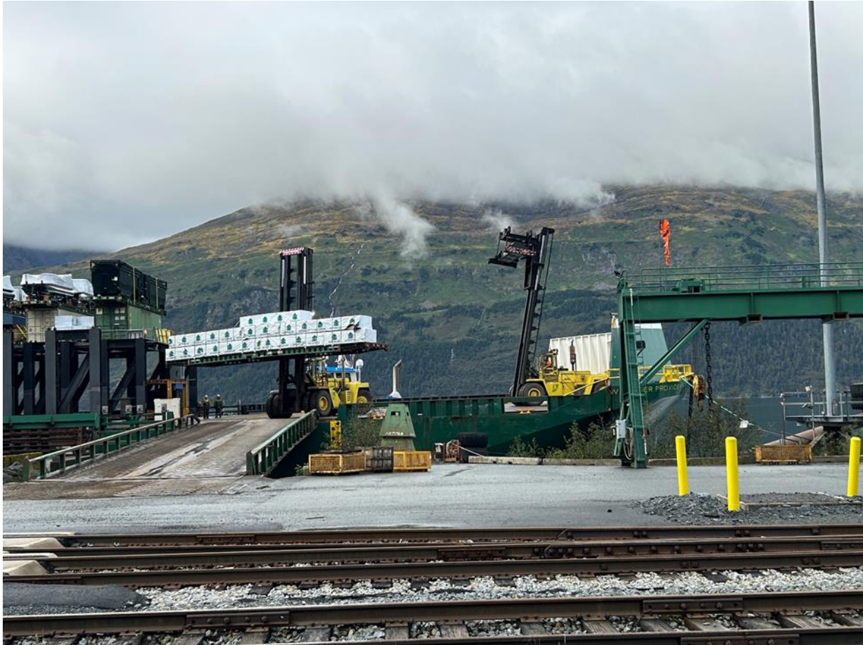
Figure 9. Alaska Marine Lines (AML) container handlers unloading containers from the bow of the barge.
