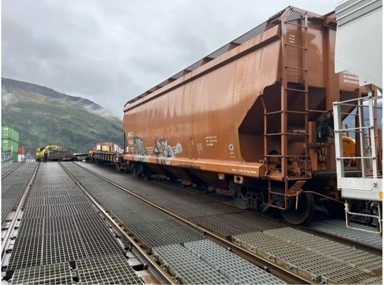
Figure 24. Rail cars being unloaded from barge to terminal via transfer ramp.
