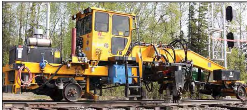
Figure 4-3 An ARRC Tie Inserter Extracts Old, and Installs New, Ties
