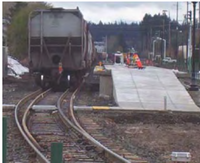
Figure 3: Freight Car on Gauntlet Track Passing Level Boarding Platform
