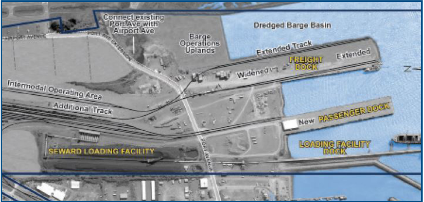
Marine terminal and upland development plans call for a widened and lengthened freight dock and port-to-airport roadway connection.
